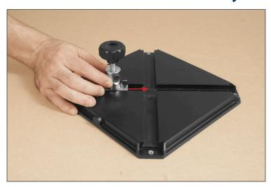
With the Ellipse Jig Base (1) centered and attached to the underside of your workpiece, insert one of the Steel Rod Guide Assembly's (2) into the center of the jig base.
