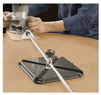
With the power turned off, move the router around the circle before turning it on to be sure that its tracking properly. Plug in the router, turn it on and slowly plunge the router so the bit cuts the full thickness of the board. Slowly work the router around the circle in the counter clockwise direction. Working the router in a counter clockwise direction keeps the router from pulling away from you while cutting. For thicker stock, you may need to make multiple depth cuts for best results..
